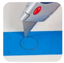
Pro Tip: Trace the outline of the penny on masking tape and cut with a utility knife. Apply tape to the boat instead of tracing on the boat.
