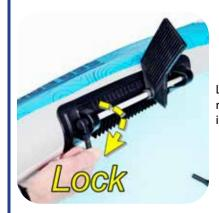
Lock the bar in place by rotating the handle down into the locking hook.
