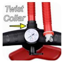
Attach a Hose To inflate the boat, attach the hose with hook-in adapter to pump handle by twisting the collar into the threaded opening until hose is tight (about 1/8 turn).
