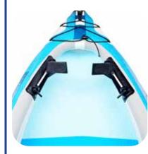
Repeat pedal installation on the other side. Pedal positions are numbered for easy alignment. Adjust pedal while on the water by lifting pedal with a foot and slide pedal fore or aft.
