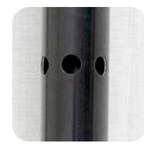
**TIP:** One shaft section has holes for feathering. By feathering the paddle, the blades are offset from each other so that when one blade is in the water, the other is at an angle to slice through the wind with little resistance.
