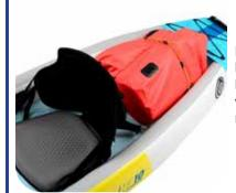
Keep heavier gear low in the boat, and keep all gear as low as possible to minimize wind resistance and to avoid making the boat top heavy.
