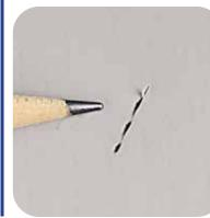
**Patching** The most common repairs are a puncture or small cut. A penny size patch is sufficient for repairs of this type.
