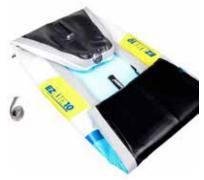
Unfold the boat until the you can see the handle. Fold the aft end towards the bow in front of the skeg base.
