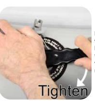
Press on center of valve tool with free hand to keep from breaking the teeth off the tool. If loosening a very tight valve, an extension tube might be needed.
